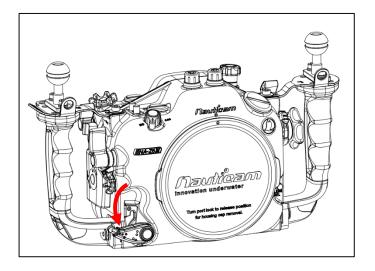
2. Gently turn the port locking lever counterclockwise to the most outward position as shown until it cannot go any further.
