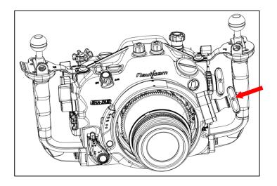
1. After install lens and gear, engage the gear on the lens by pushing the knob inwards, then turn the knob both direction to check if the lens is functioning.
