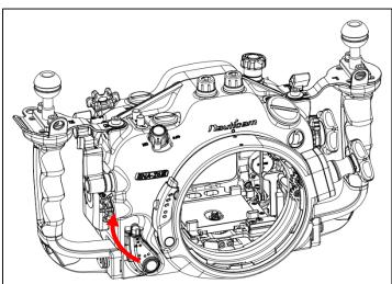
Lock the housing port locking lever into place by turning the lever to the inward lock position. It comes with a click sound indicating the extension ring is locked in position.
