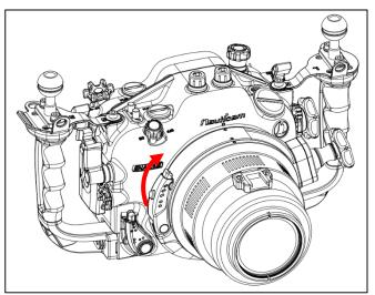
5. Lock it into place by turning the locking lever to the inward lock position and when a "click" sound is heard.
