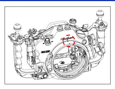
4. Prepare the sealing O-ring first as instructed on page 3, align the extension ring "o" mark with housing's, and push the product onto the housing gently.
