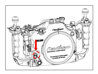
1. Gently push the safety button of housing port locking lever downwards.
