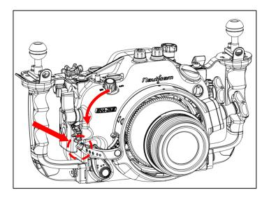
3. Then press the extension ring lock safety button and turn the locking lever to release position as shown.
