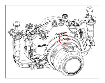
4. Align the alignment "O" mark of the extension ring and the port, gently push the port into the extension ring until it cannot go in any further.
